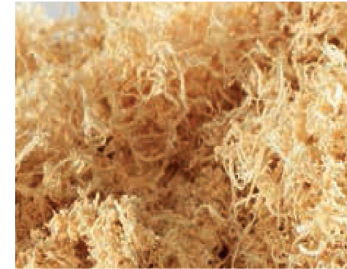
Competitor's sanding dust shows evidence of fibre ripping.
