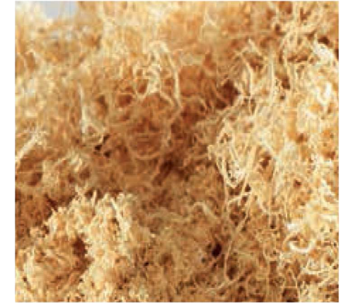
Competitor's sanding dust shows evidence of fibre ripping.
